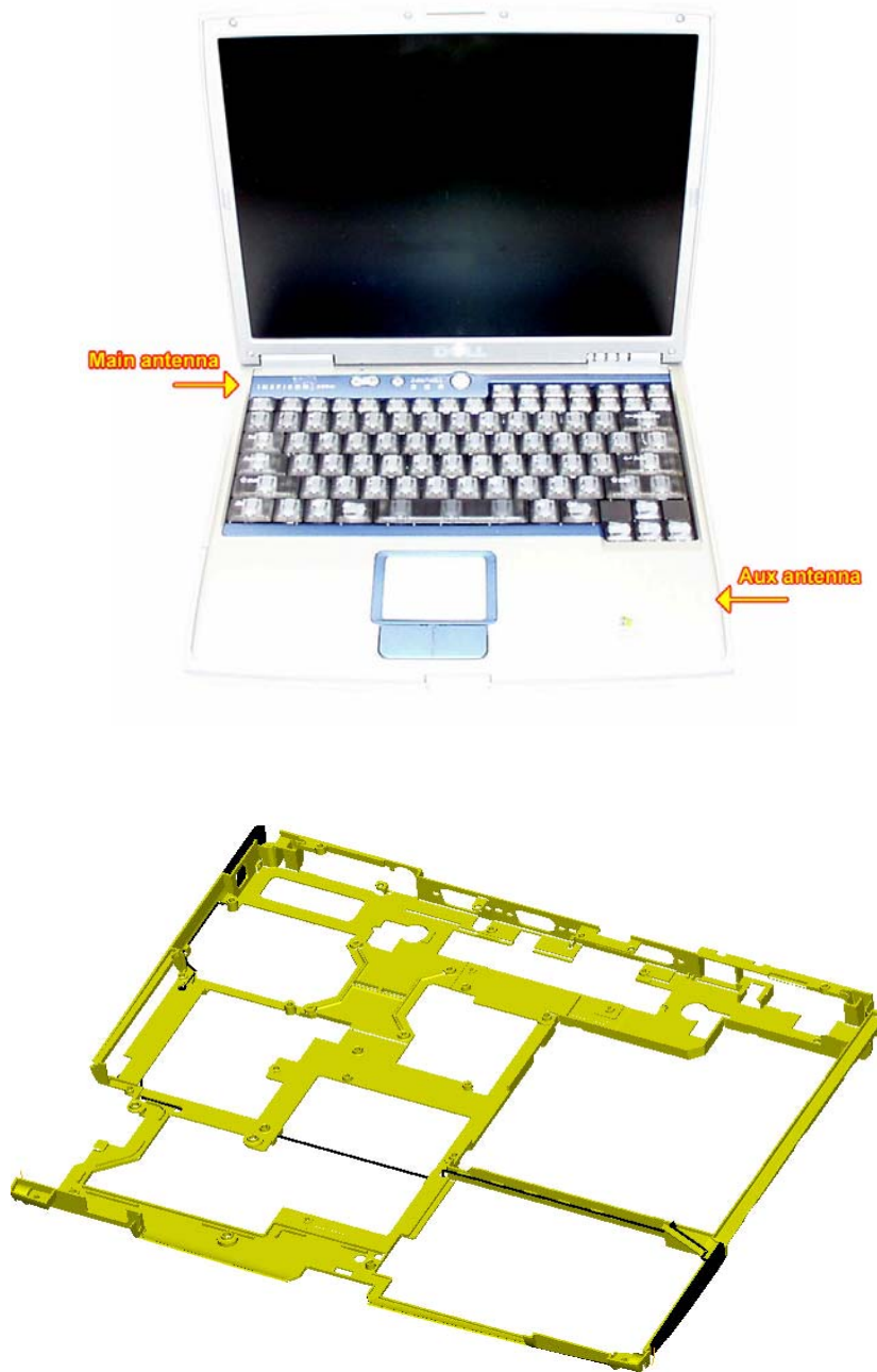
< Dell Latitude Laptop PC (M/N: PP05L) – MAIN and AUX antenna location and cable routing >
