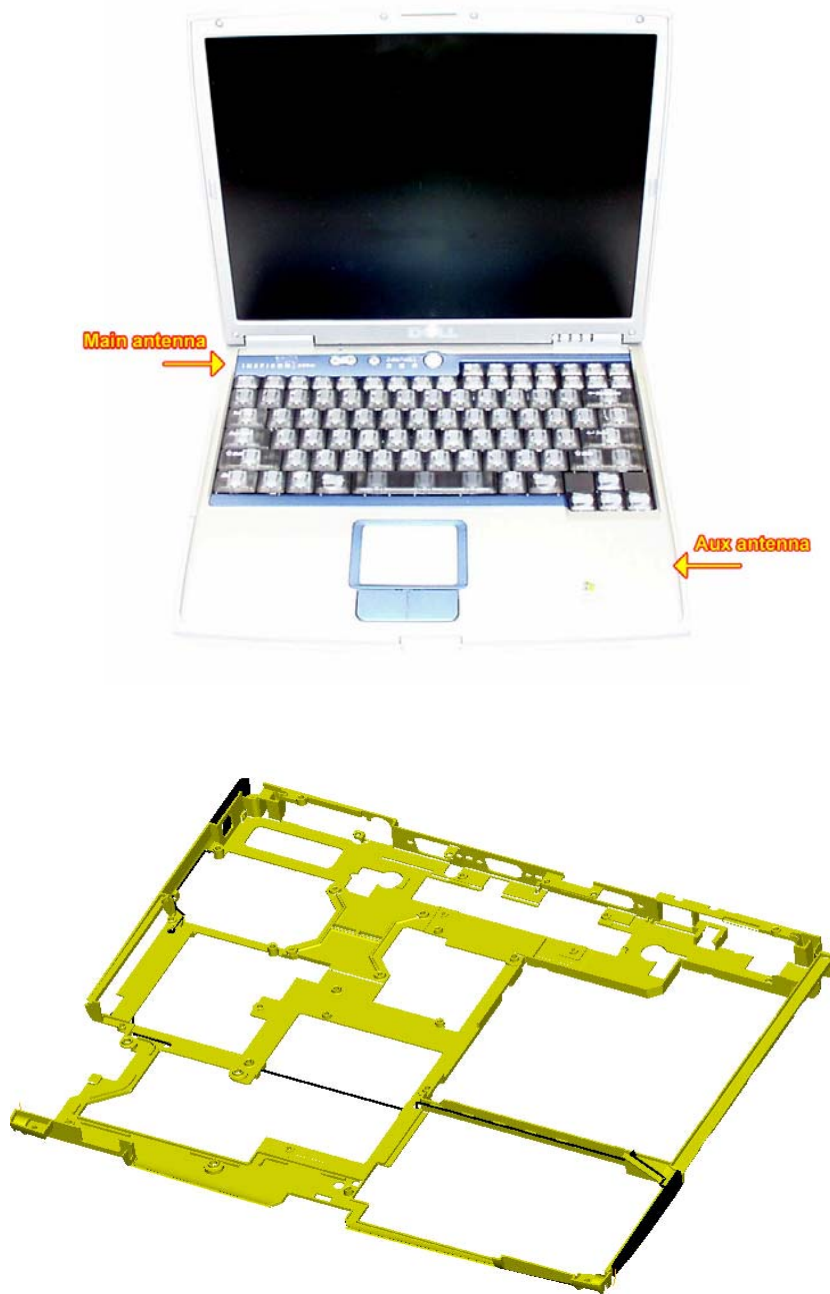
< Dell Latitude D600 (M/N: PP05L) – main and aux antenna location and cable routing >
