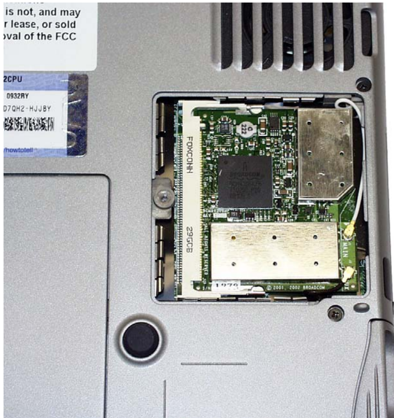
< D.U.T. installed in miniPCI slot >
