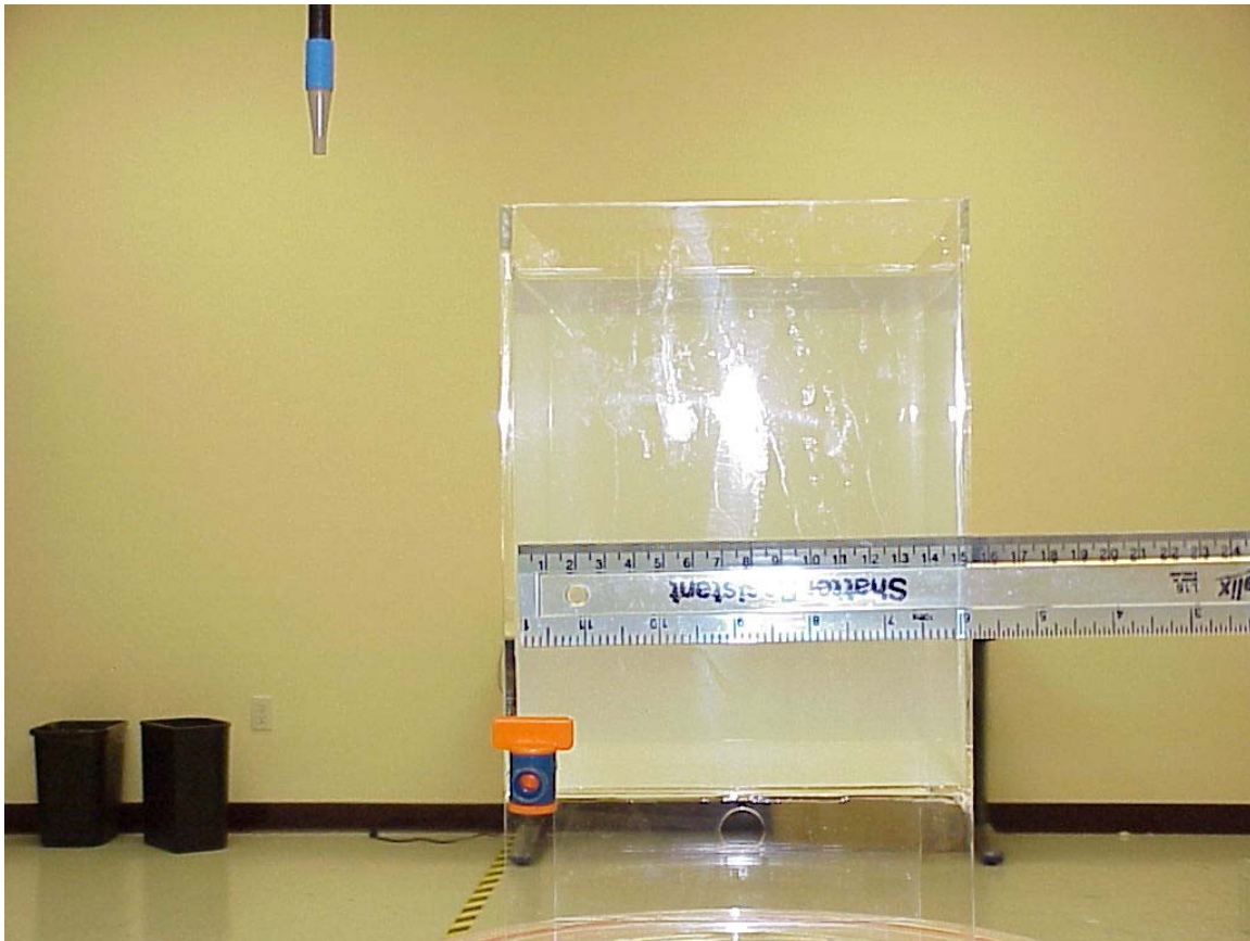
Photo 6. Photo to demonstrate 15 cm Z-axis flat phantom
