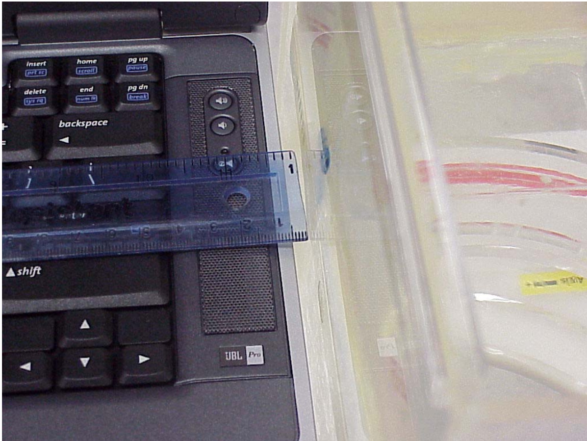
Photo 7. Right antenna bystander position distance
