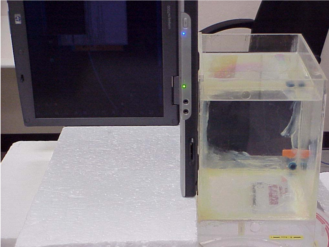
Photo 11. Left antenna lap position
