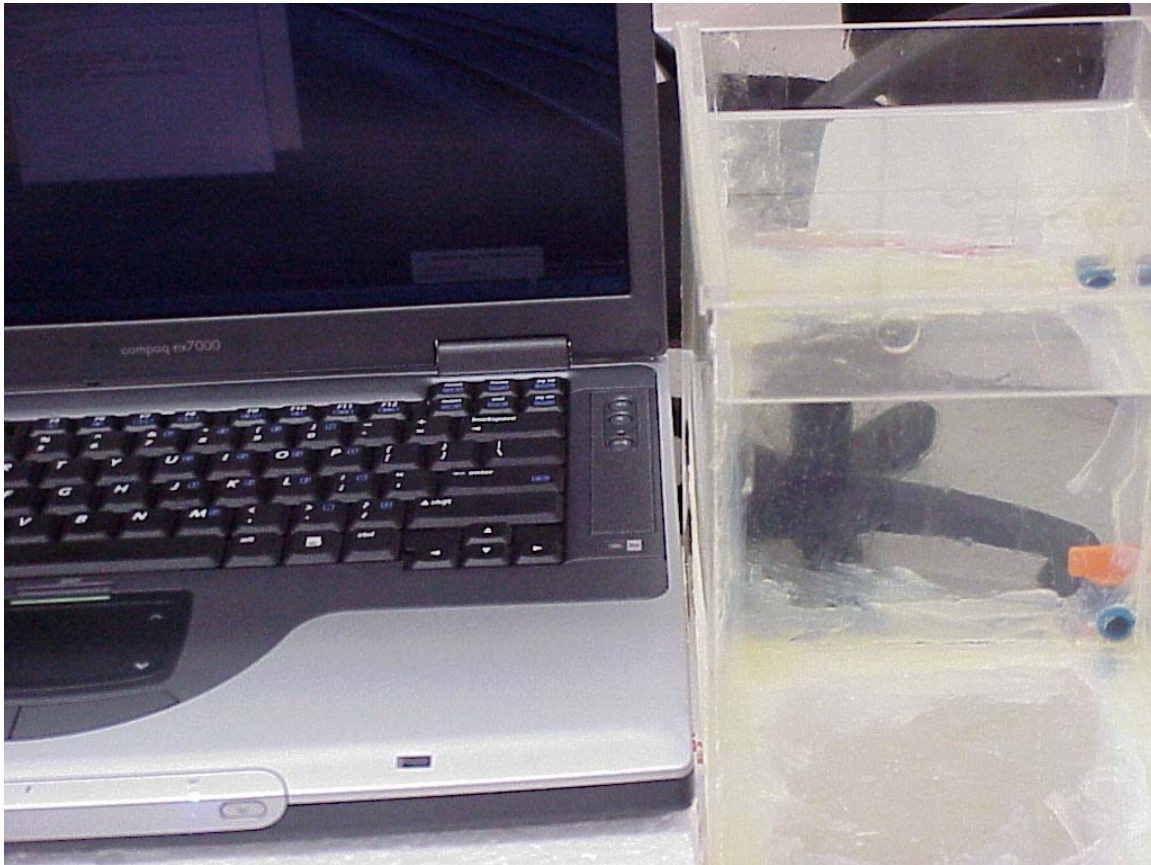
Photo 6. Right antenna bystander position
