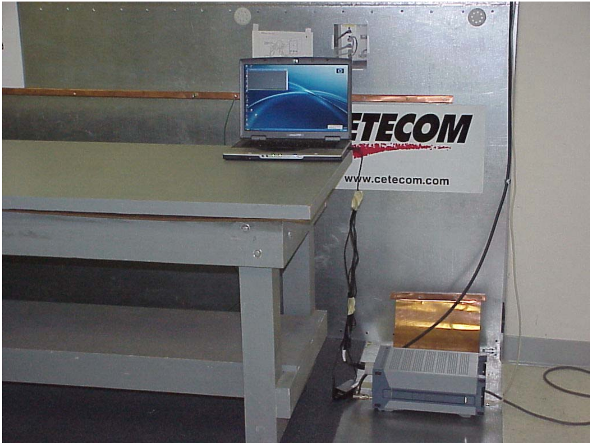
Test set-up – AC Line conducted emissions
