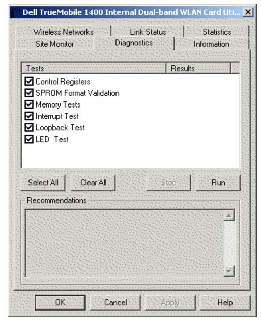
6. If your **Dell TrueMobile WLAN Card** fails any of the diagnostics tests, see the Troubleshooting section.
