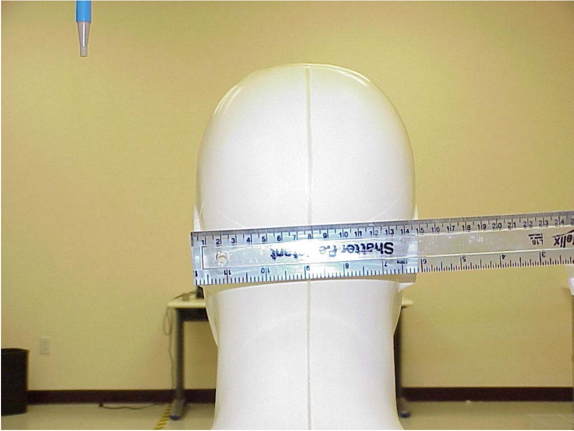
Photo 6. Photo to demonstrate 15 cm Z-axis head phantom
