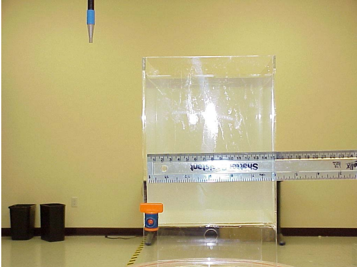
Photo 7. Photo to demonstrate 15 cm Z-axis flat phantom
