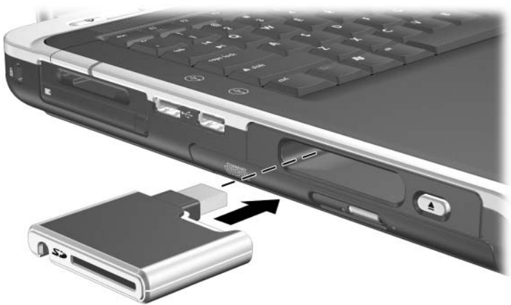
Inserting the Digital Drive in the Digital Bay
