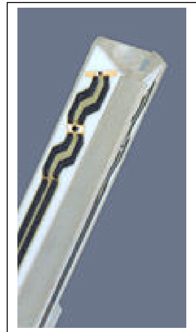
Inside view of ET3DV6 E-field Probe
