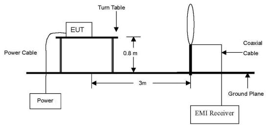
The diagram below shows the test setup that is utilized to make the measurements for emission from 30 \( \mathref{M} \) to 1 \( \mathref{M} \) Emissions.
