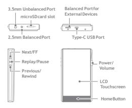
**3.5mm Unbalanced Port:** Connects to the earphones and the headphones with 3.5mm unbalanced ports.
