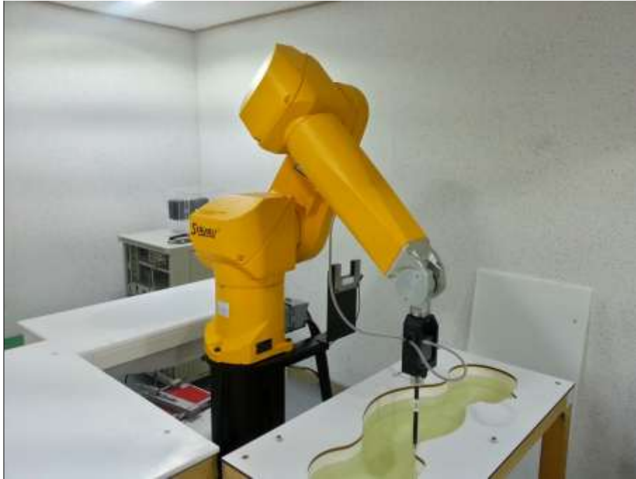
Photograph of the SAR measurement System
