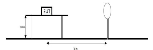
The diagram below shows the test setup that is utilized to make the measurements for emission from 30 Mz to 1 Gz emissions.
