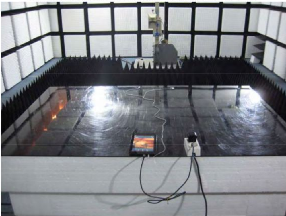
Radiated Emissions Above 1 GHz - Rear View(Play mode)
