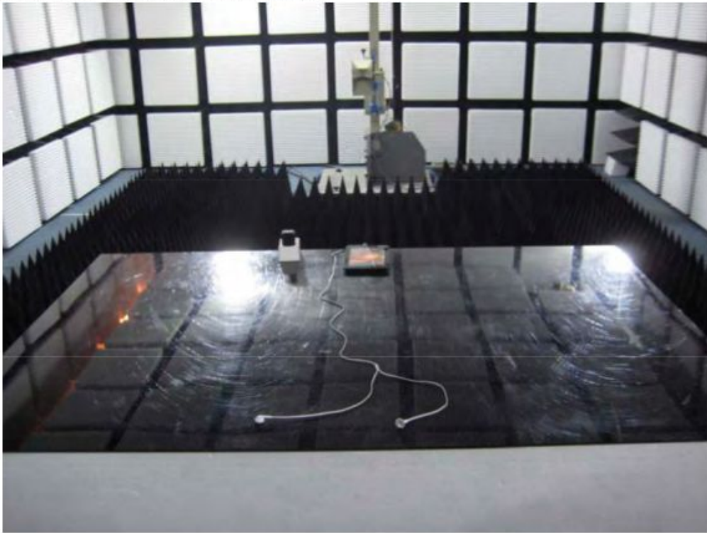
Radiated Emissions Above 1 GHz- Front View(Play mode)
