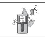
Promptly turn the power of the product off and disconnect the AC connector from the power outlet if the product produces smoke, smells, or unusual sounds. Using the product in abnormal conditions may cause fire or electric shock.
