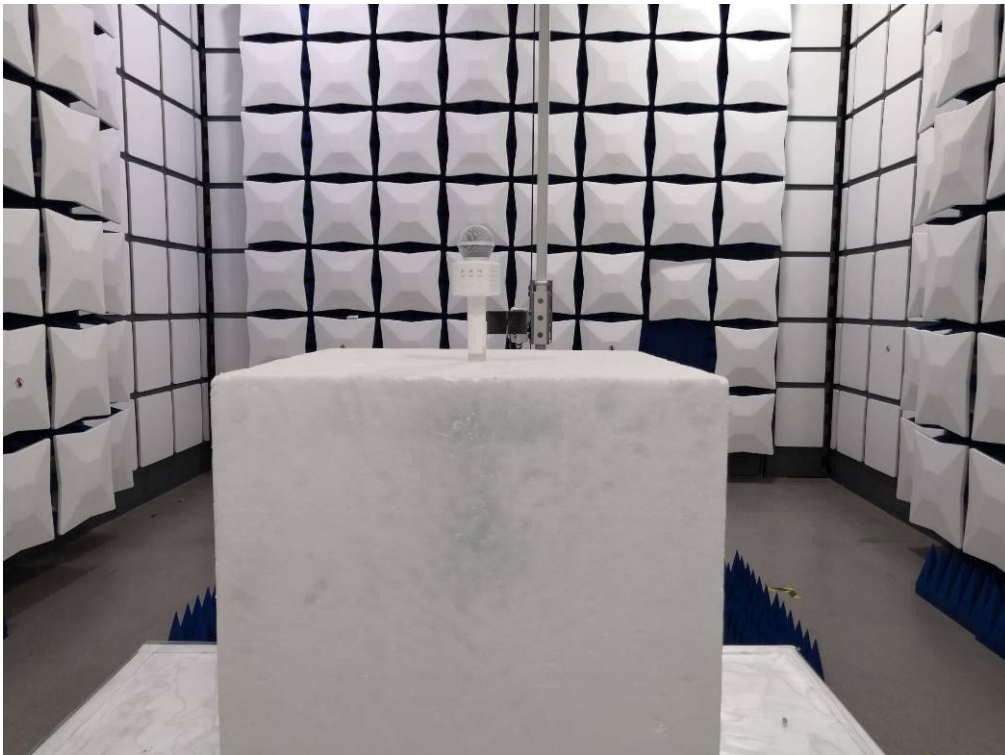
RADIATED EMISSION TEST SETUP ABOVE 1GHZ
