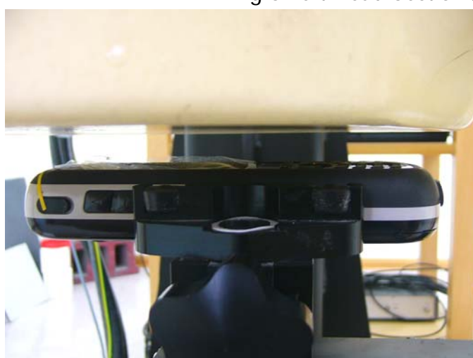
Fig.7 Body worn- EUT front to flat phantom (testing in GPRS Mode)
