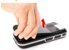
4. Lift the end portion of the battery pack and completely detach it from the device.
