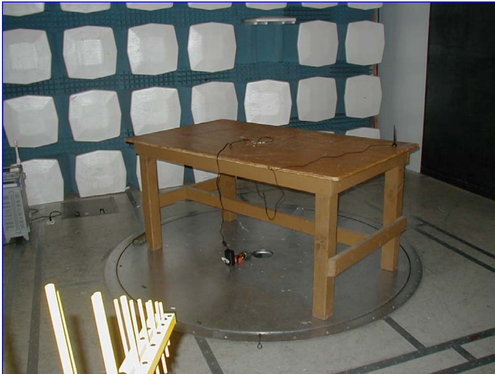
Photograph 1. Radiated Emission Limits Test Setup
