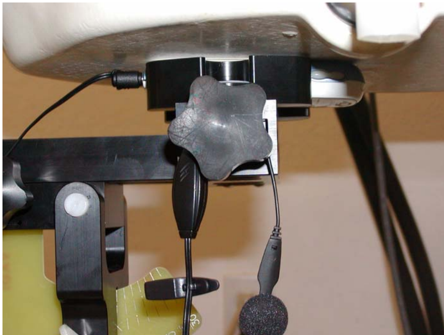
Bottom Touching Phantom with Earphone – Side View
