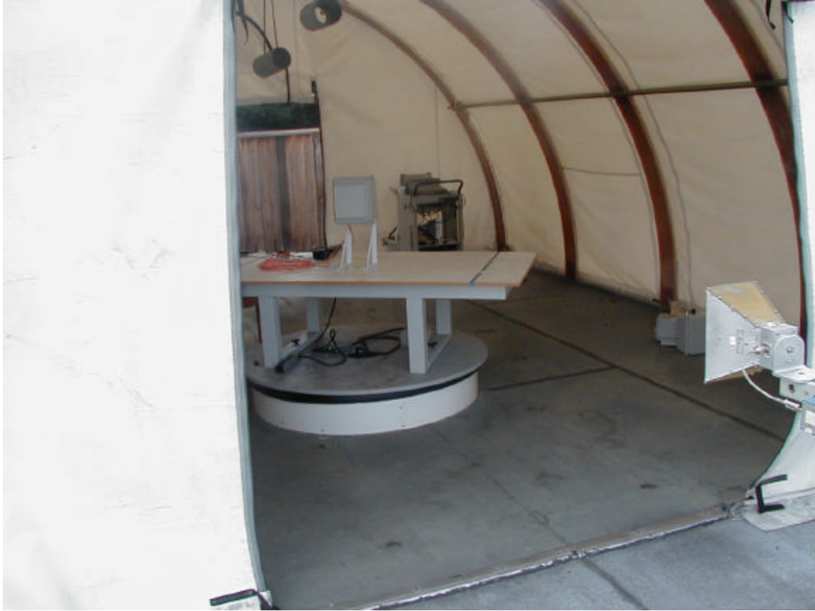
Radiated Emission above 1 GHz Test Setup
