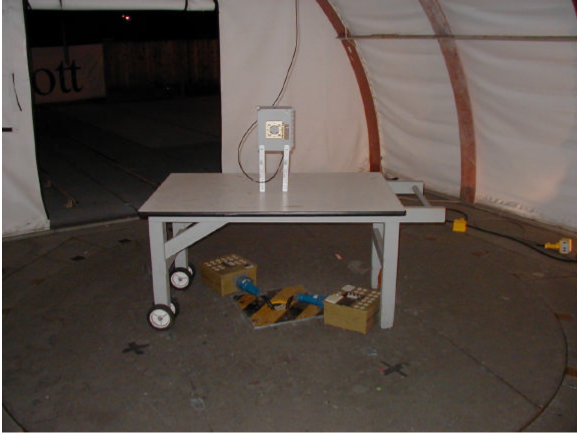
Radiated Emission Below 1 GHz Test Setup
