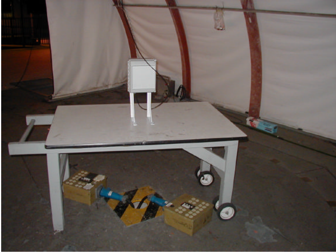
Radiated Emission Below 1 GHz Test Setup
