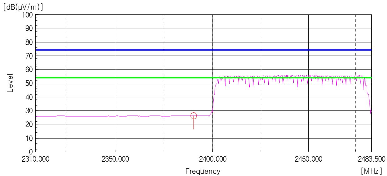
Peak Detector: RBW: 1 MHz, VBW: 1 MHz (2 483.5 MHz - 2 500.0 MHz), Worst case (High, Vertical)
