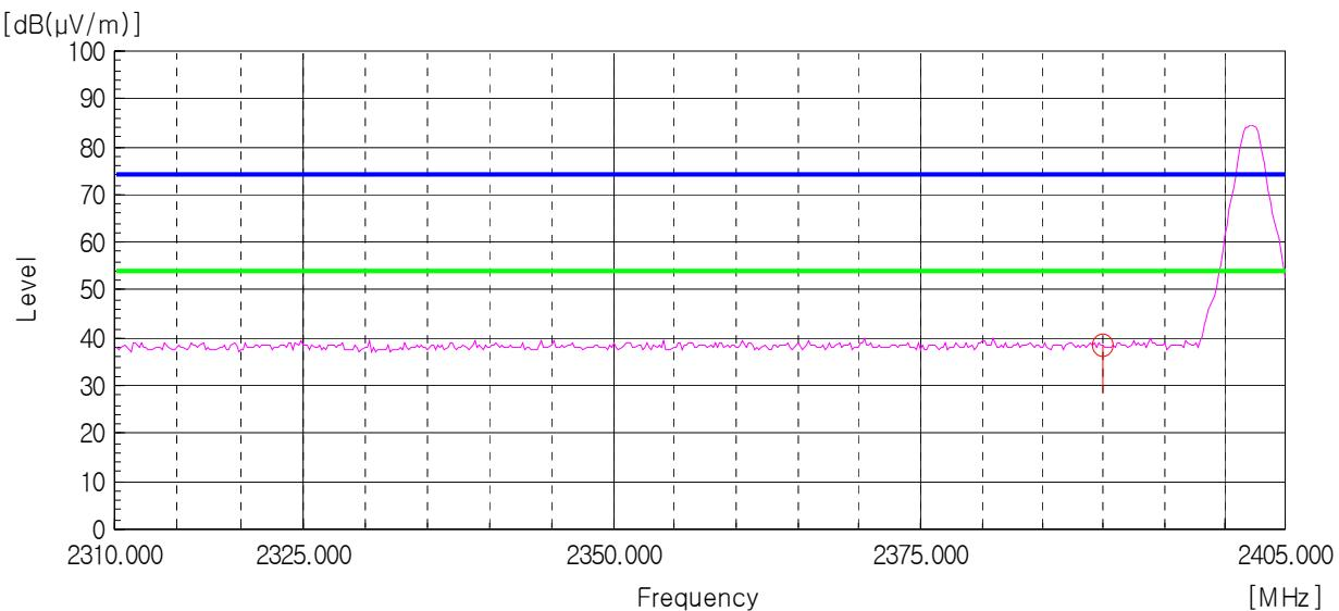
AV Detector: RBW: 1 MHz, VBW: 10 Hz (2 310 MHz - 2 390 MHz), Worst case (Low, Vertical)
