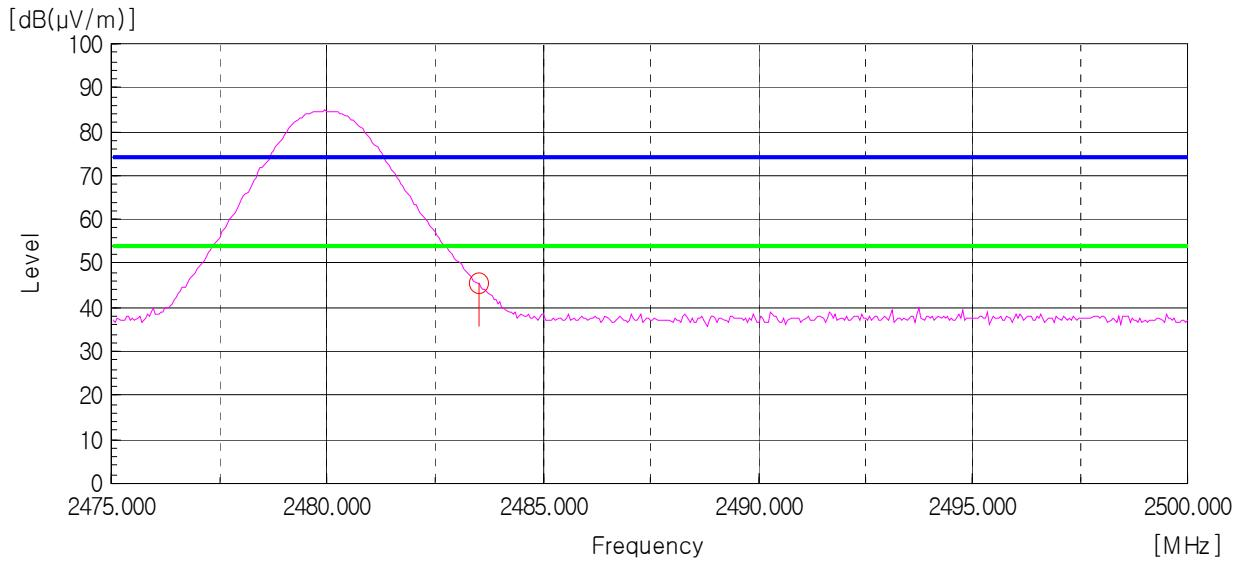
AV Detector: RBW: 1 MHz, VBW: 10 Hz (2 483.5 MHz - 2 500.0 MHz), Worst case (High, Vertical)
