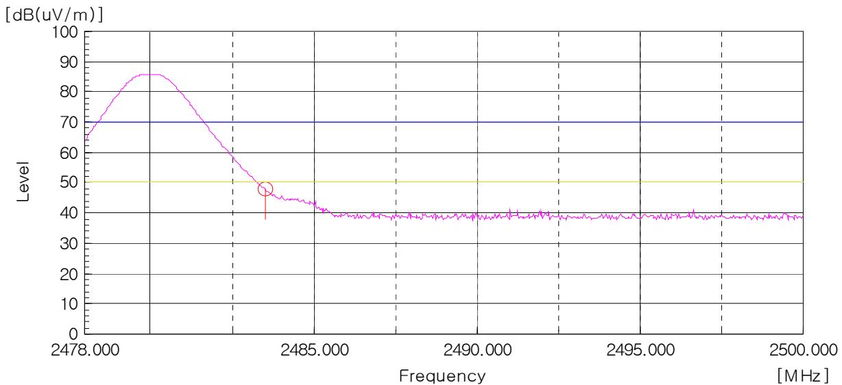
AV Detector: RBW: 1MHz, VBW: 10 Hz (2 478.0 MHz - 2 500.0 MHz), Worst case (High, Horizontal)
