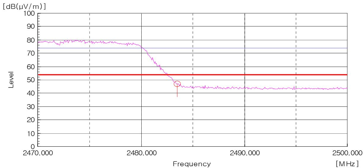
AV Detector: RBW: 1MHz, VBW: 10 Hz (2 483.5 MHz - 2 500.0 MHz), Worst case (High, Vertical)
