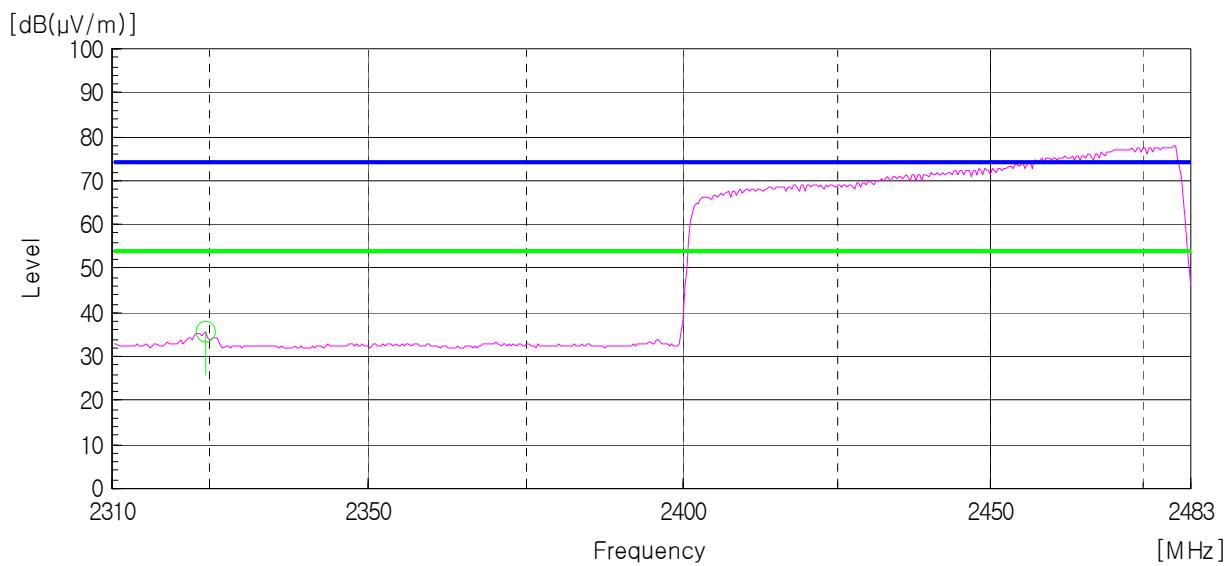
Peak Detector: RBW: 1 MHz, VBW: 1 MHz (2 450.0 MHz - 2 500.0 MHz), Worst case (High, Horizontal)
