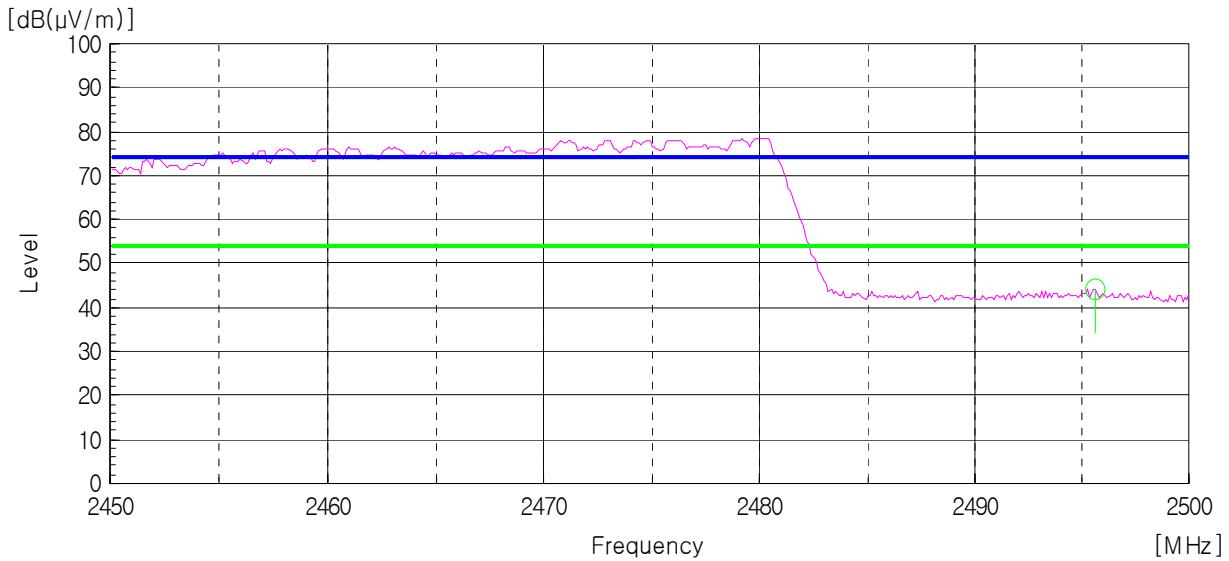
AV Detector: RBW: 1 MHz, VBW: 10 Hz (2 475.0 MHz - 2 500.0 MHz), Worst case (High, Horizontal)
