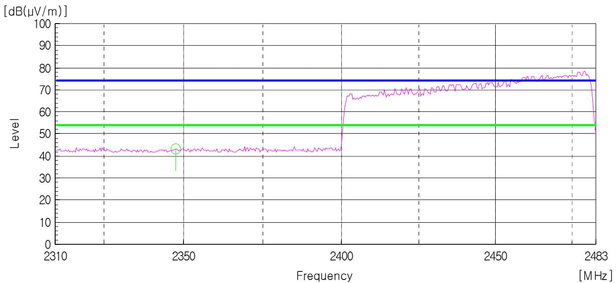
AV Detector: RBW: 1 MHz, VBW: 10 Hz (2 310 MHz - 2 405 MHz), Worst case (Low, Horizontal)
