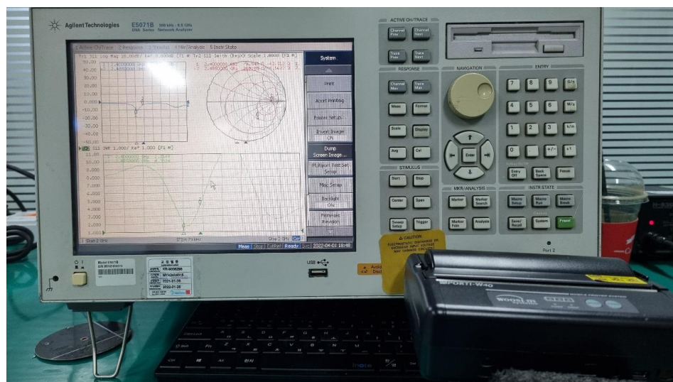
Figure 4.2.1 Test by network analyzer
