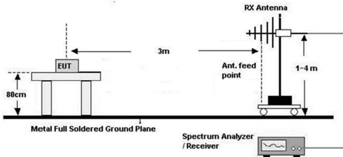
**Test Procedure of Receiver Spurious Emissions (Below 1GHz)**
