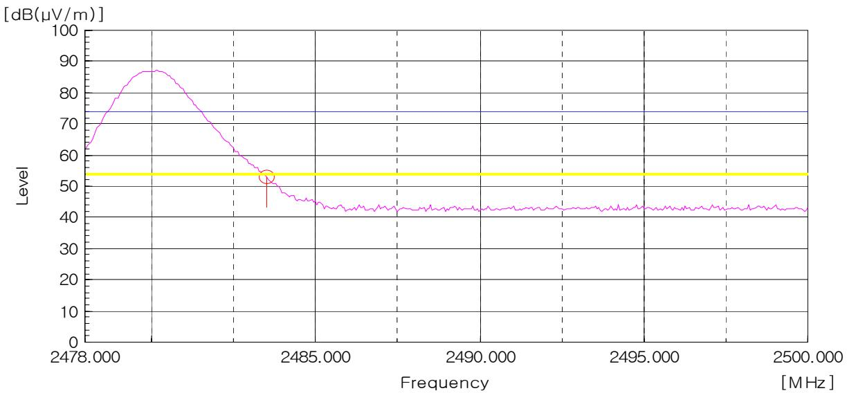
AV Detector: RBW: 1MHz, VBW: 10Hz (2 483.5 MHz – 2 500 MHz), Worst case (High, Vertical)
