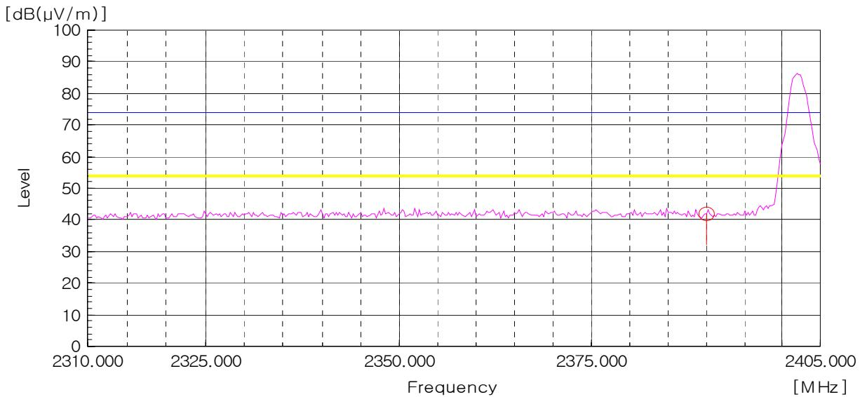
AV Detector: RBW: 1 MHz, VBW: 10 Hz (2310 MHz – 2390 MHz), Worst case (Low, Vertical)
