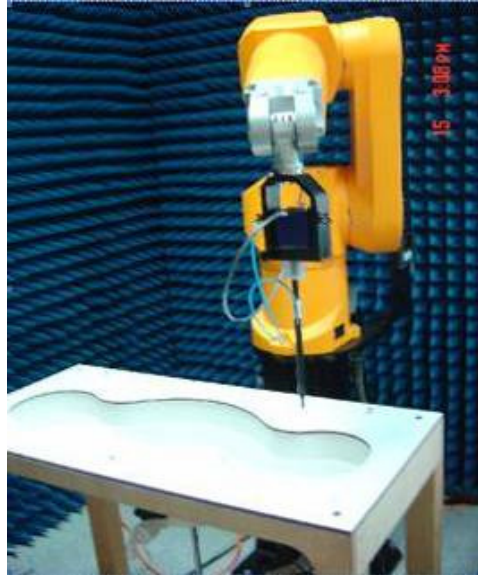
Photo 1: SAR measurement System
