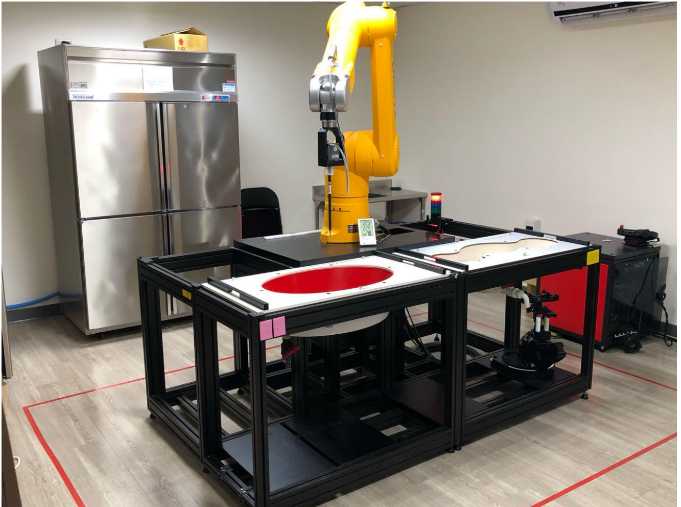
Liquid depth in the flat Phantom ( \geq 15\text{cm} depth) HSL(2450MHz)
