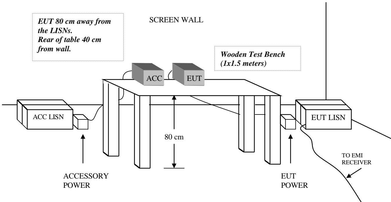
**FIGURE 2: PLOT MAP & LAYOUT OF TEST SITE
