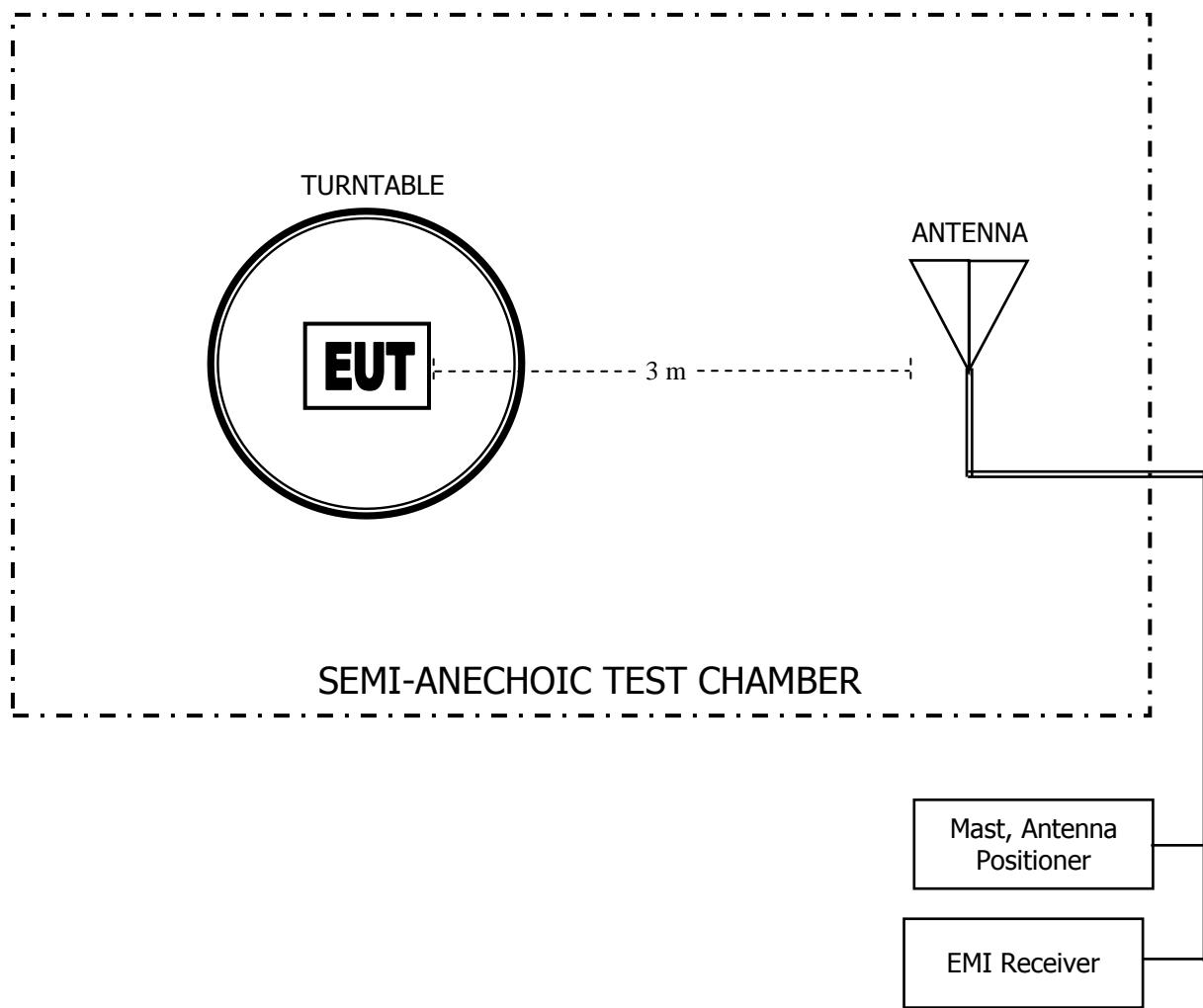
**FIGURE 3: PLOT MAP & LAYOUT OF TEST SITE
