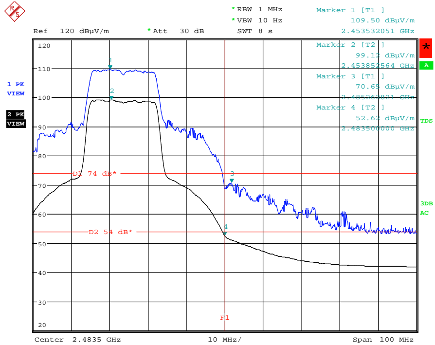
Figure 70: Radiated Emissions at Band Edge, Spectral Diagram, IEEE 802.11n (20MHz), Channel 10 (2457MHz)
