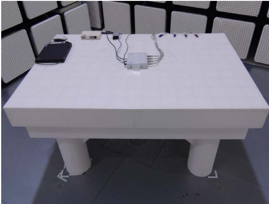
Photograph 4: Set-up for Radiated Emission of Transmitter, Front View
