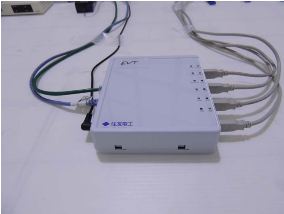
Photograph 6: Set-up for Radiated Emission, EUT Configuration X-Axis
