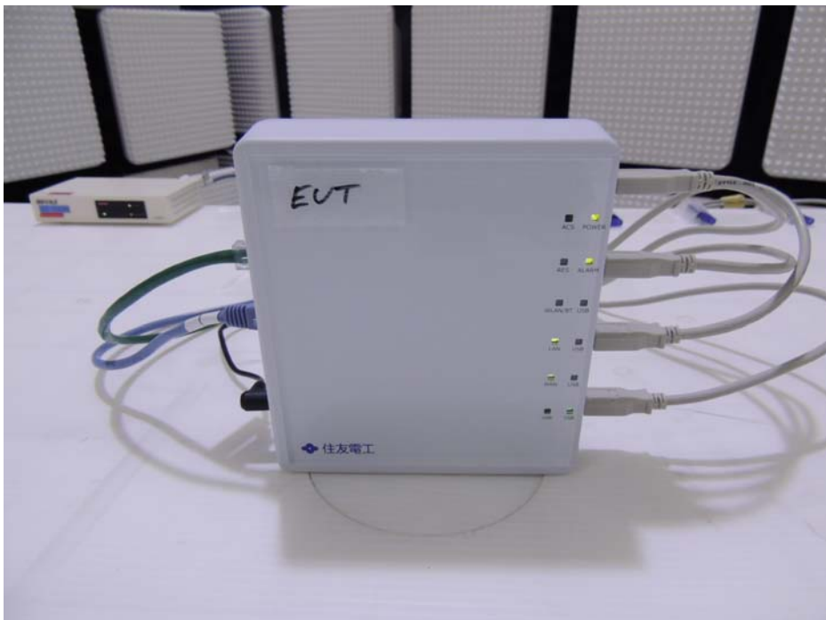
Photograph 7: Set-up for Radiated Emission, EUT Configuration Y-Axis
