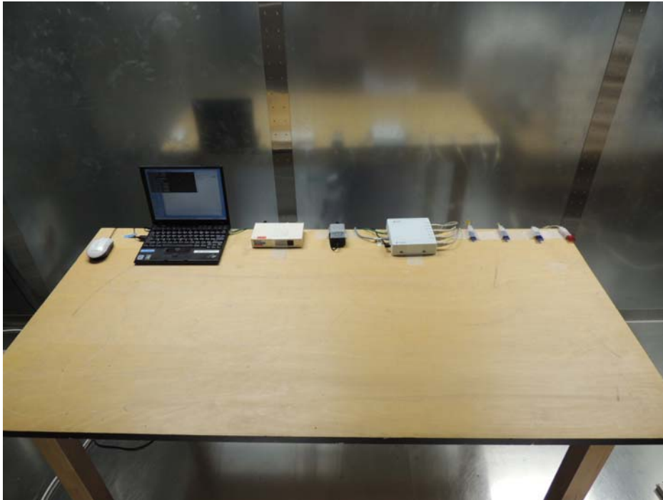
Photograph 2: Set-up for AC Power Line Conducted Emission of Transmitter, Front View
