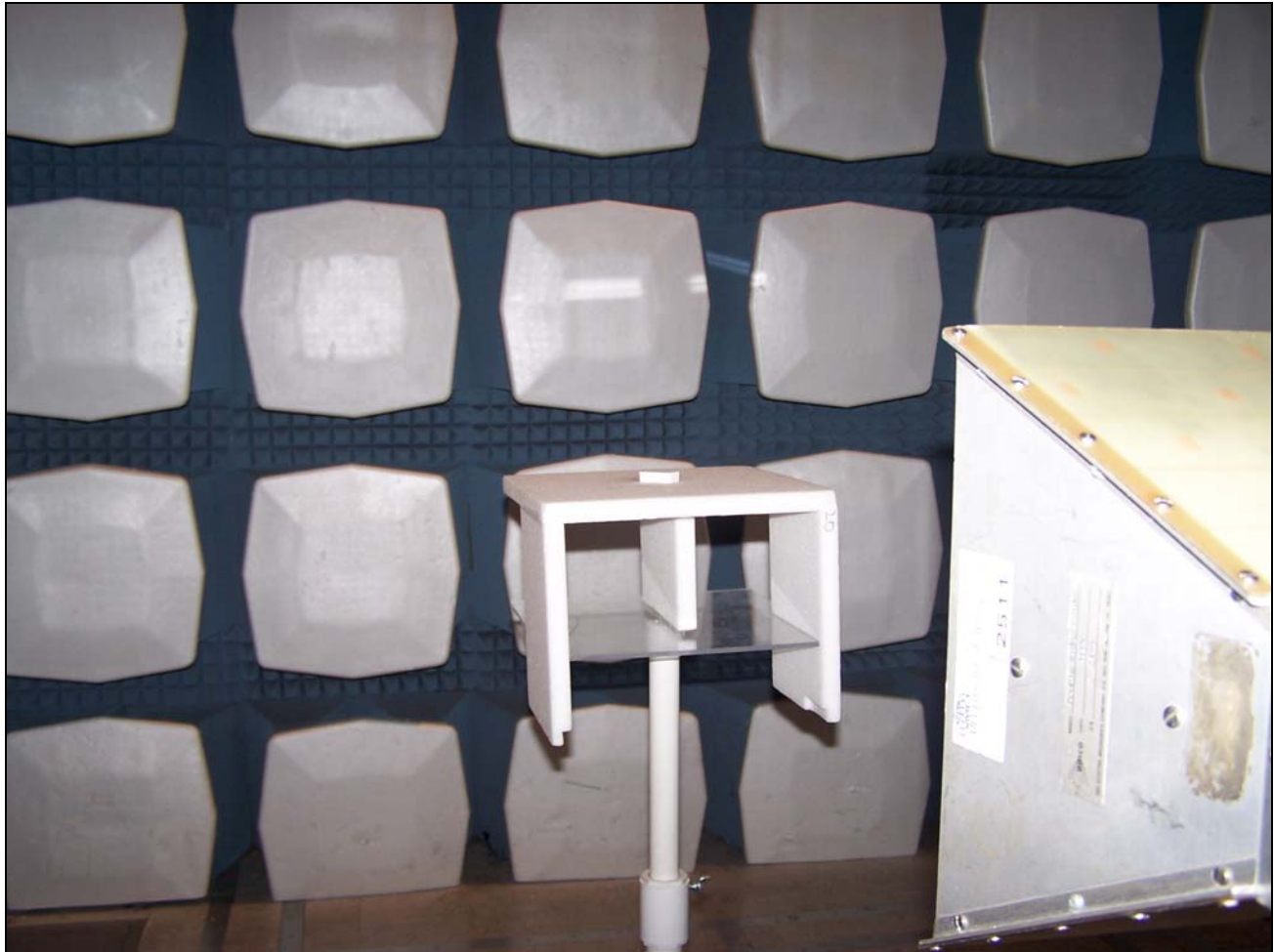
Photograph 2. 15.250(d)(1) Radiated Emissions Above 960 MHz (RMS Average), Test Setup
