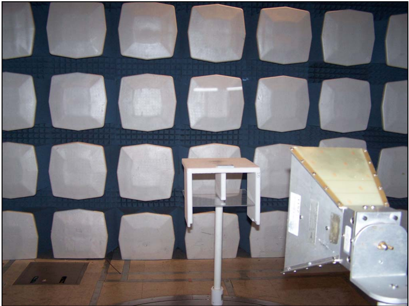
Photograph 1. -10 dB Bandwidth, Test Setup
