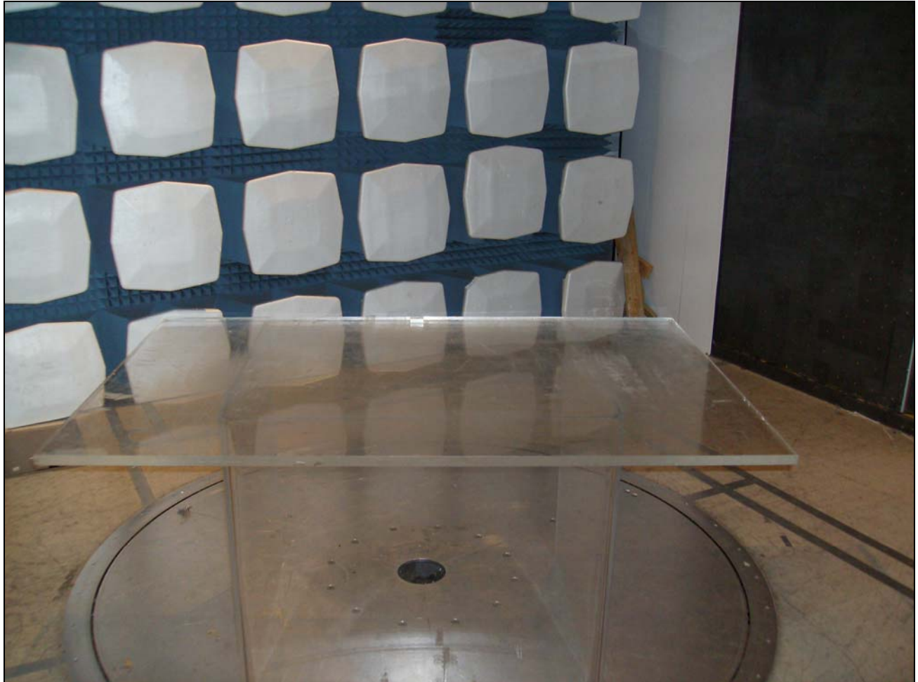
Photograph 3. Radiated Emission Limits Test Setup
