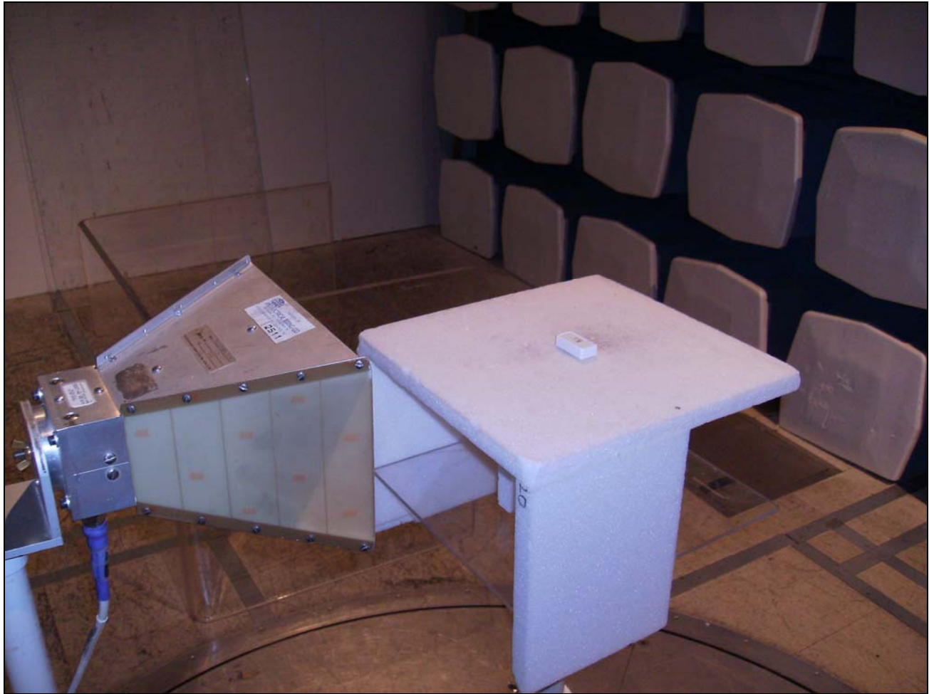
Photograph 1. -10 dB Bandwidth, Test Setup
