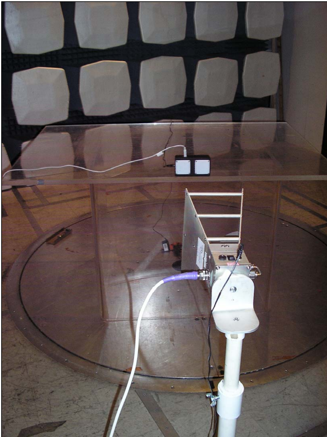
Photograph 2. -10 dB Bandwidth Test Setup
