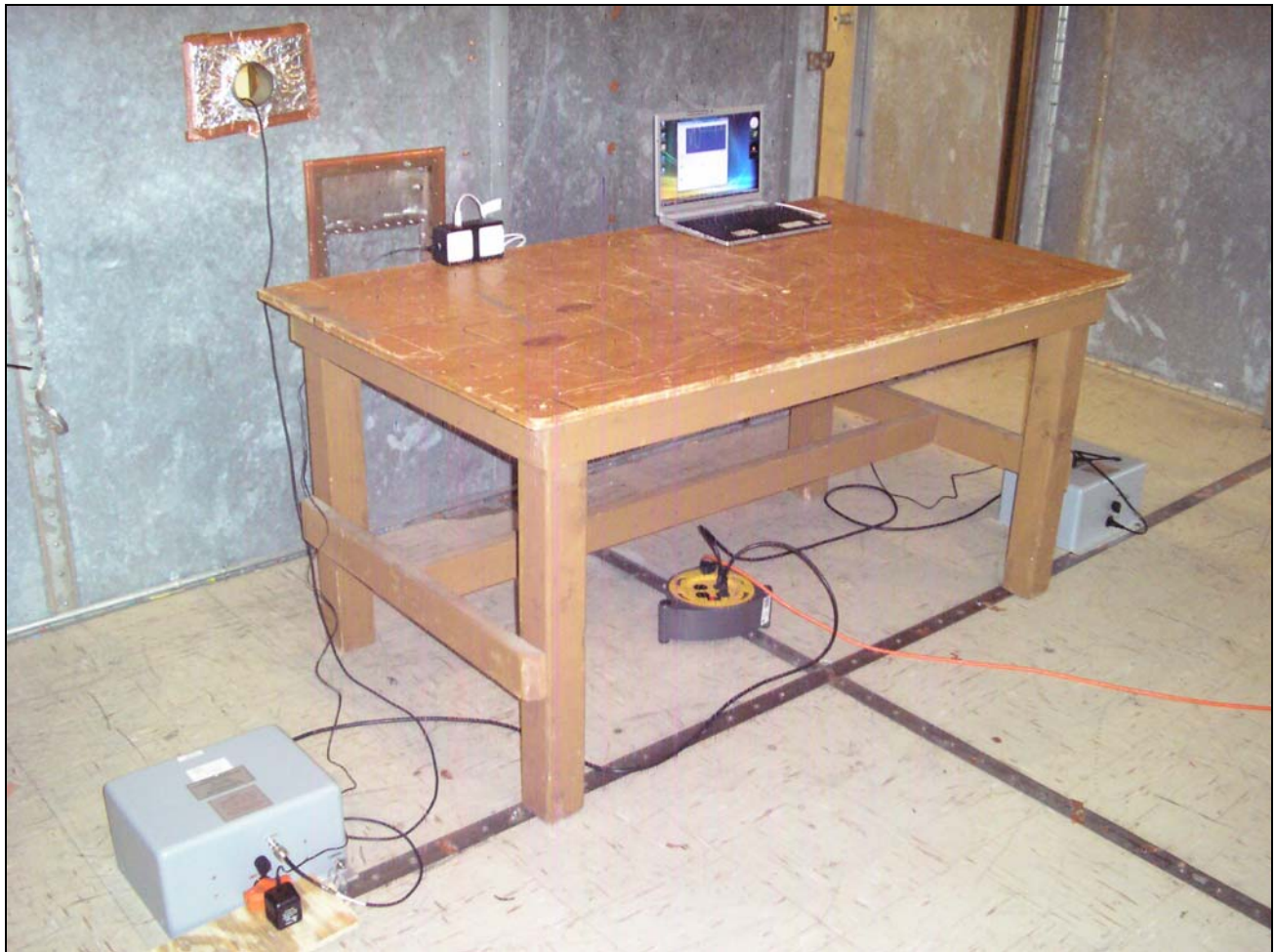
Photograph 1. Conducted Emissions Test Setup
