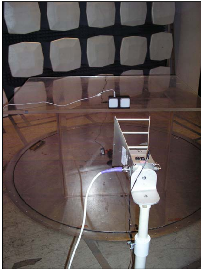
Photograph 5. Peak Radiated Emissions Requirements Test Setup
