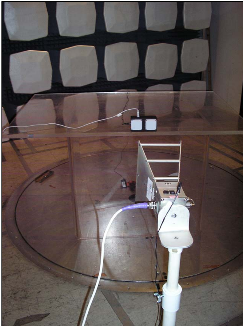
Photograph 4. Average Radiated Emissions Requirements, Narrowband Test Setup
