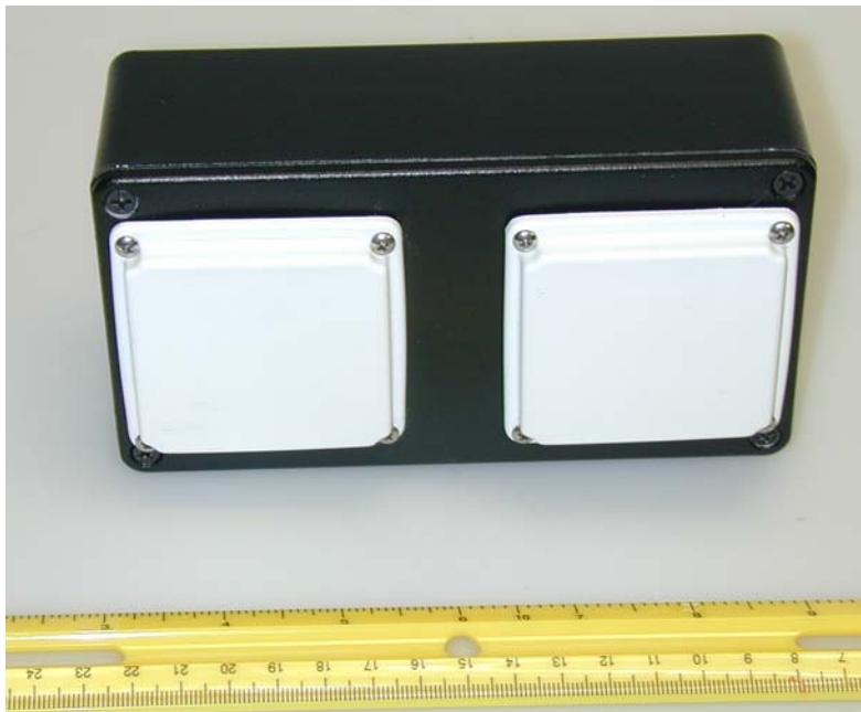
Figure 1. Radar Developer's Kit – Lite (RaDeKL) Unit with Identical Dual Antennas, One for Transmit and the Other for Receive
