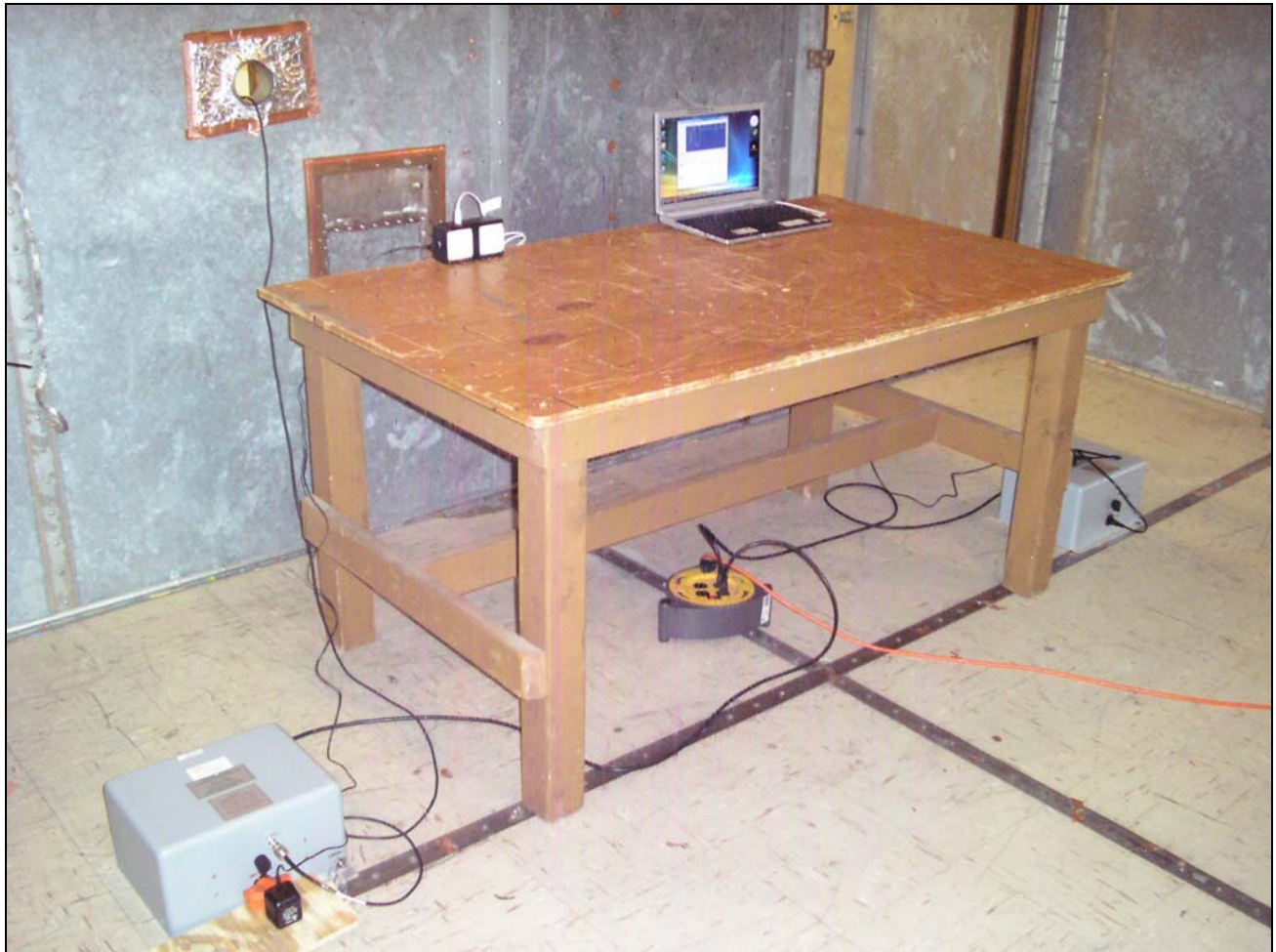
Photograph 3. Conducted Emissions, Test Setup
