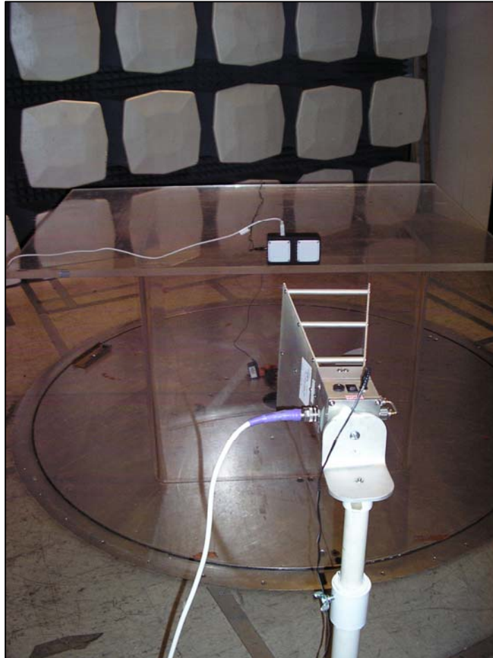
Photograph 4. -10 dB Bandwidth, Test Setup
