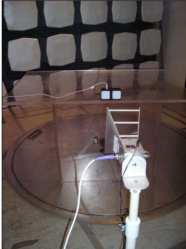
Photograph 7. Peak Radiated Emissions Requirements, Test Setup
