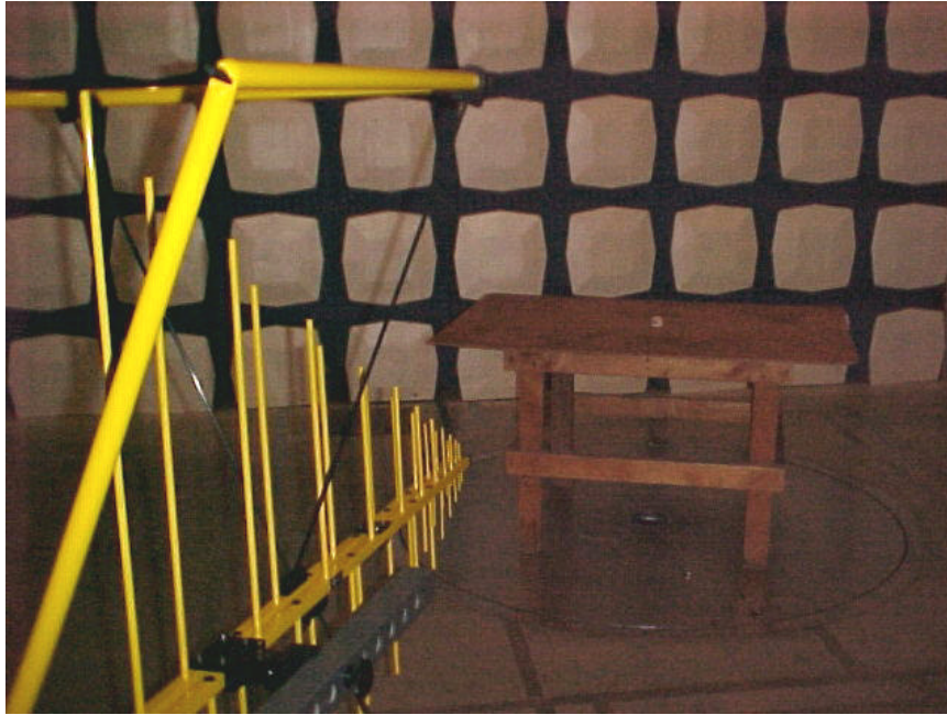
Figure 1. FCC Intentional Radiators Test Setup Photo
