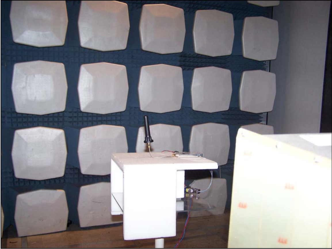
Photograph 1. Radiated Emissions, Test Setup
