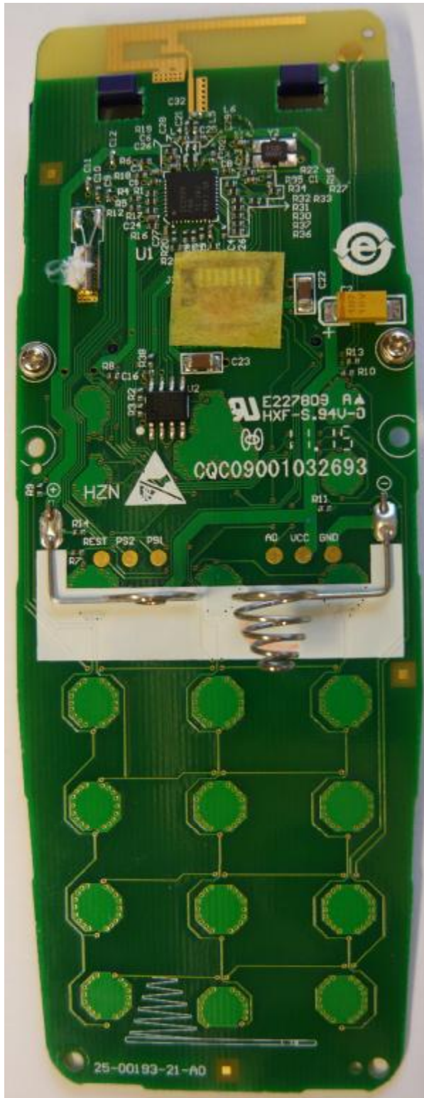
Bottom of PCBA as viewed with back cover removed. PCBA is removed from front cover.
