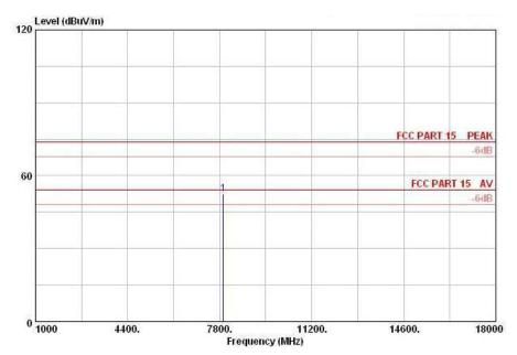
Dis. / Ant. : 3m Ant. pol. : HORIZONTAL Limit : FCC PART 15 Env. / Ins. : 23\*C/54\* Engineer : Jamy\_Yu : Receiver M/N:03-00181 : DC 5V From PC EUT
