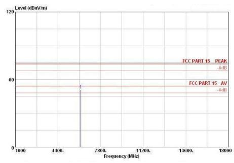
Dis. / Ant. : 3m Ant. pol. : VERTICAL : FCC PART 15 Limit Env. / Ins. : 23\*C/54% EUT : Receiver M/N:03-00181 Engineer : Jamy\_Yu
