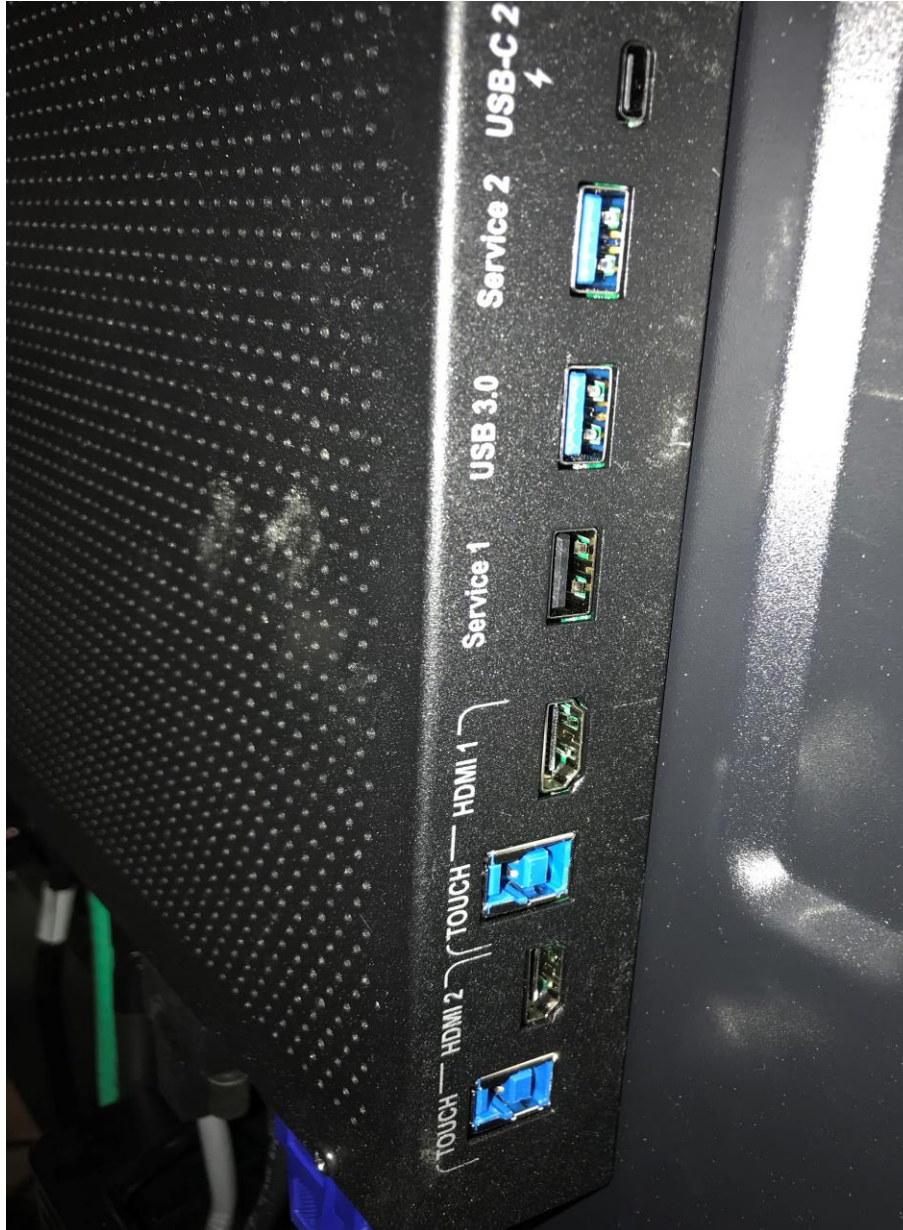
SIDE CONNECTOR (Scalar Board - Baseband PCB)
