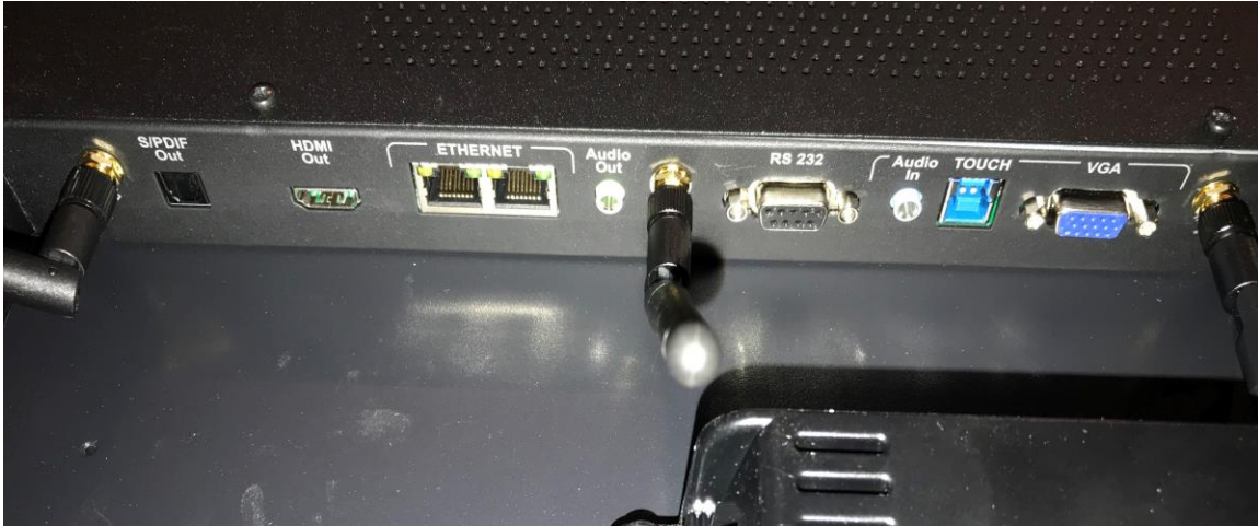
BOTTOM CONNECTORS (Scalar Board - Baseband PCB)
