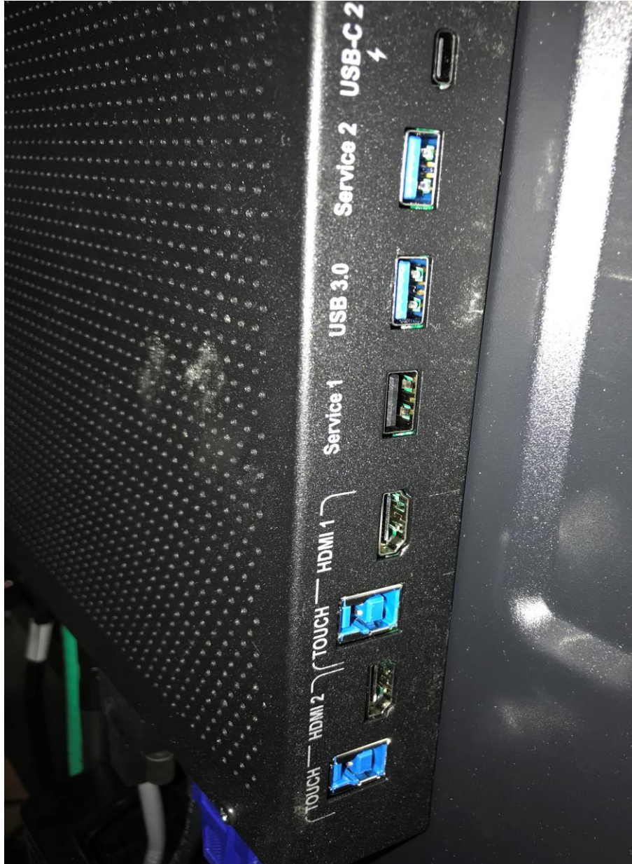
SIDE CONNECTOR (Scalar Board - Baseband PCB)
