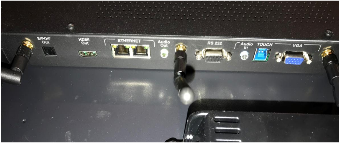
BOTTOM CONNECTORS (Scalar Board – Baseband PCB)
