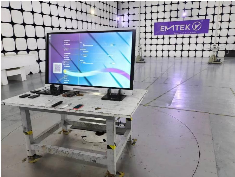
Spurious Emission Test Setup (Above 30MHz)
