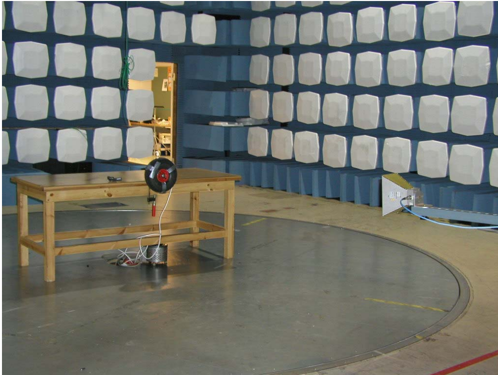
Photograph 1. Radiated disturbance emission test
