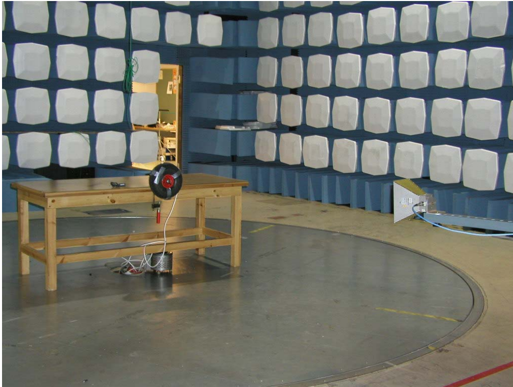
Photograph 1. Radiated disturbance emission test
