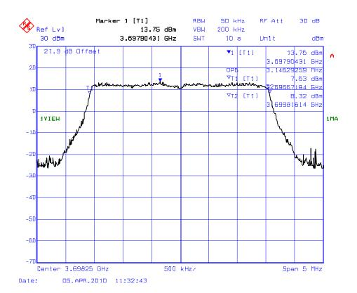
Plot # 6: 99% Occupied Bandwidth Center Freq.: 3696.50 MHz, Ch Spacing: 7.0 MHz
