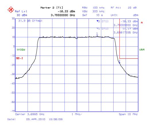
Plot # 8: Conducted Band-edge Emissions (Upper Band Edge) Center Freq.: 3698.25 MHz, Ch. Spacing: 3.5 MHz
