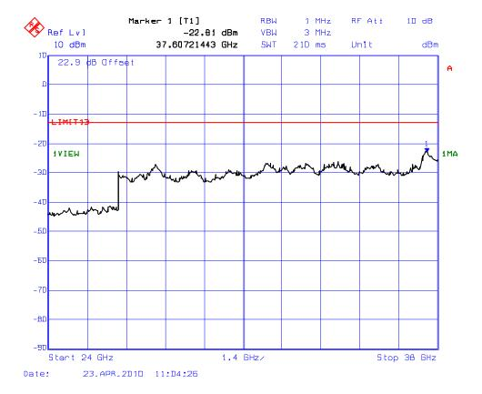
Plot # 10: **Transmitter Conducted Spurious Emissions** Center Freq.: 3696.50 MHz, Ch. Spacing: 3.5 MHz, High-Power
